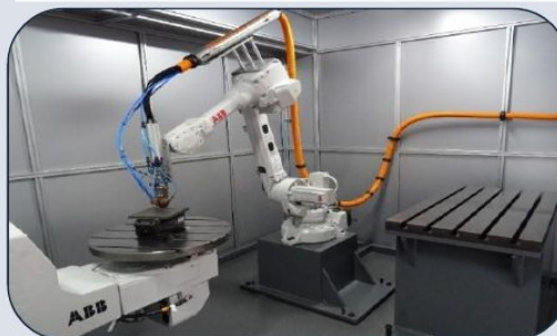
Robotic Laser Cladding Machine for Valve Seat
